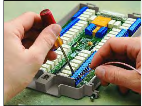
Screw terminals use oversized connectors for easier, mistake-free wiring. Easy-to-use removable terminals are available on some models.
